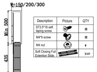
STEP2:Install the slide on the side board by 6pcs
