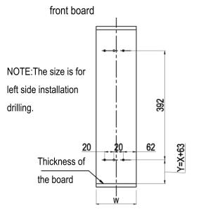
STEP1:Drilling 6pcs Φ2.5 hole on the cabient
