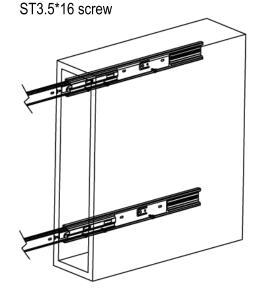
STEP4:Drilling 6 pcs  $\Phi2.5$  hole on the
